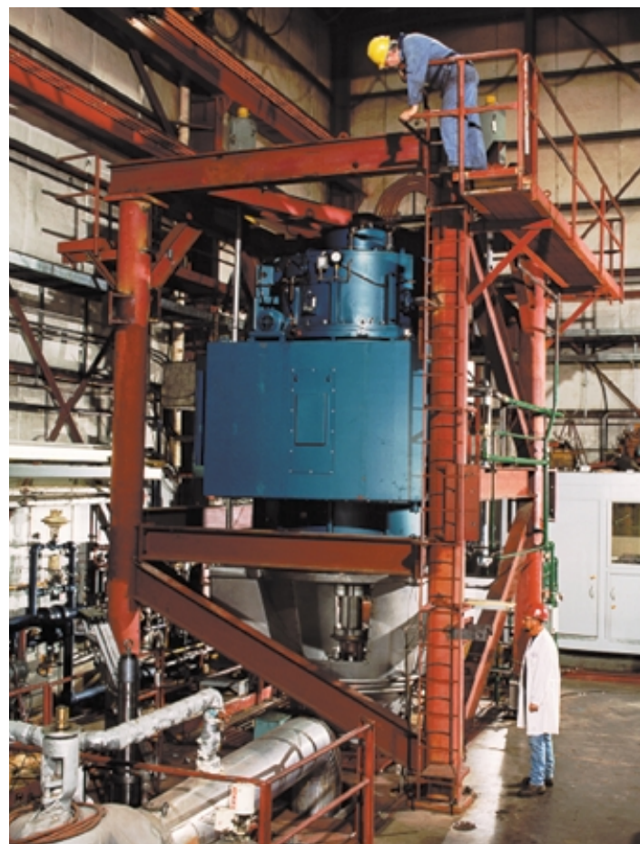
3 ■ Providing for the North American market, Sulzer's test facility in Burnaby, British Columbia, Canada, is state of the art. The test rig is designed for high-energy pump testing in both 50- or 60-Hertz configurations.
