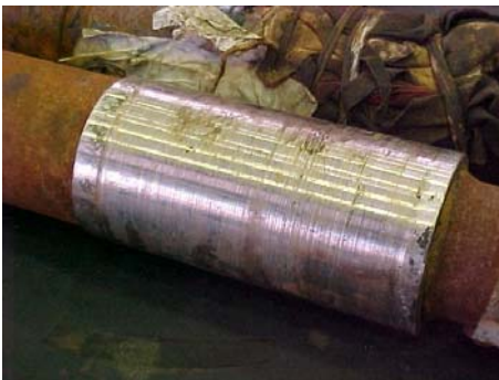
Worn bearing sleeve
