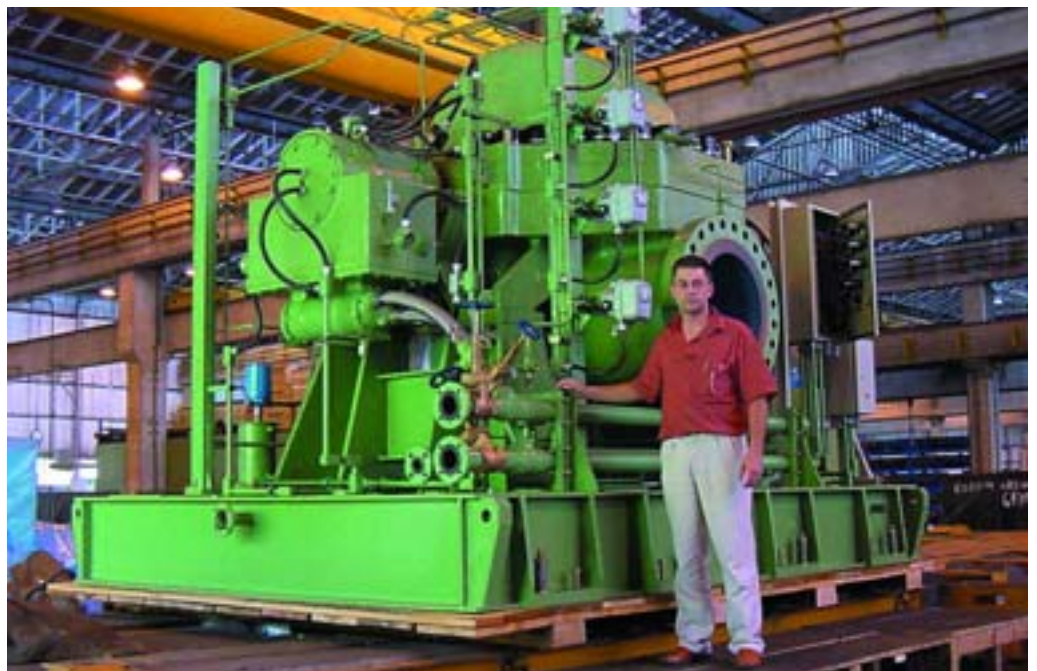
1 The HPDM 600-940-s+s/30 pump produces around 9 MW of power. The finished casing weighs 26 tons, and consists of a horizontally divided casing that is held together with studs.
