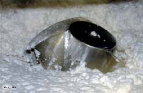
1 Pulper in a paper mill: the material handled in the pulp and paper industry can have a high solid matter content. Sulzer Pumps is a full-line supplier of products to meet all medium-consistency pumping requirements.
