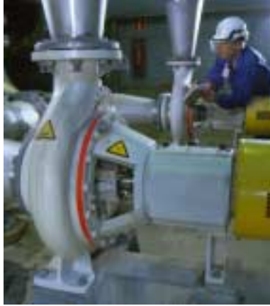
Figure 4. AHLSTAR™ APP Process Pump with ready-fitted double mechanical seal (dead-end).
