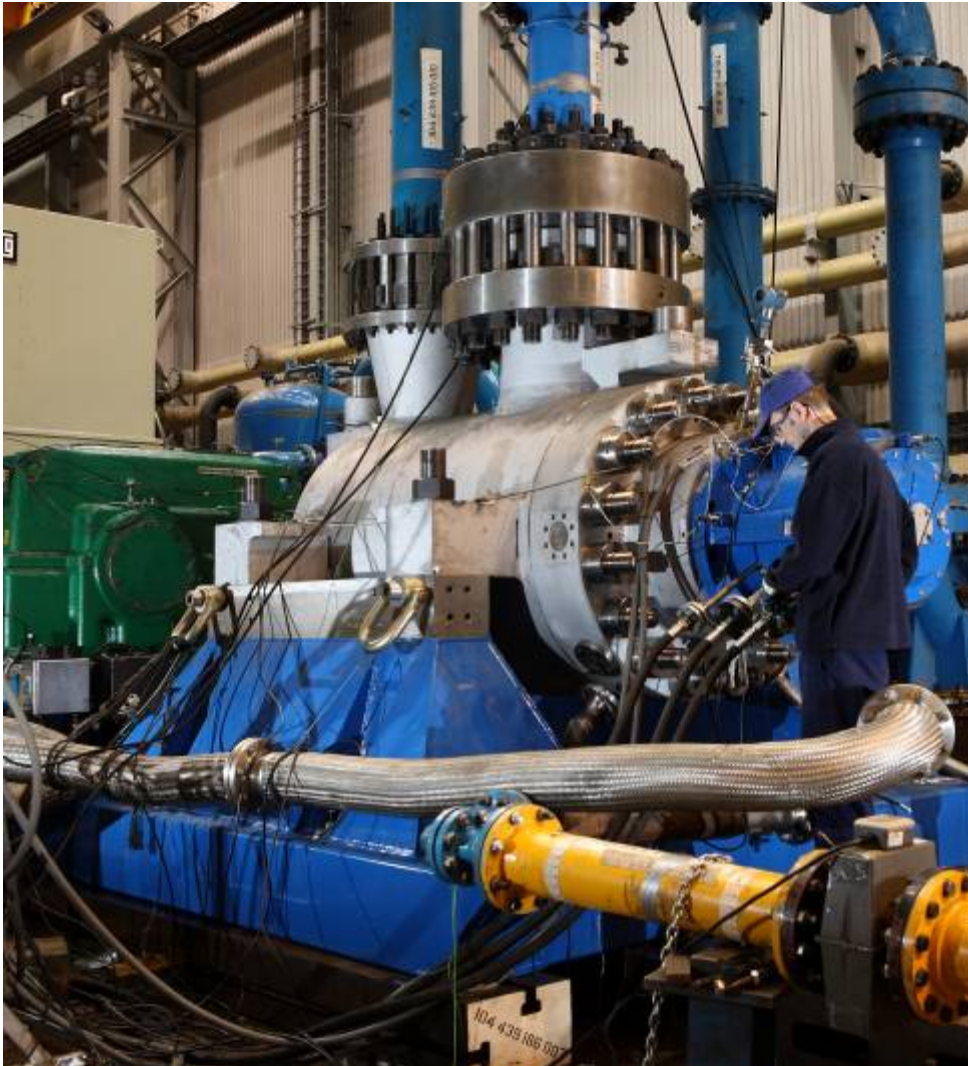
Sulzer boiler feed pump similar to those sold by the Glasgow office undergoing performance testing
