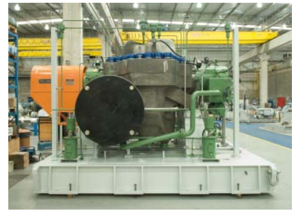
HPDM s+s water transport pump
