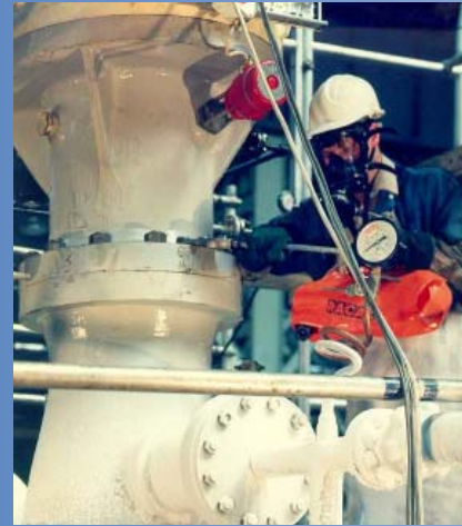
Cryogenic pumping requires special sealing solutions for reliable operation
