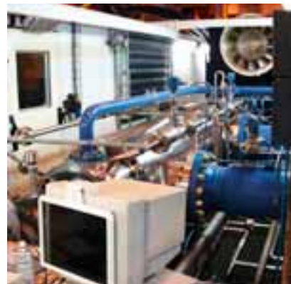
Pumps are tested on Sulzer's testbed simulating actual conditions.
