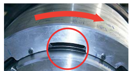
Cover locked and secured
