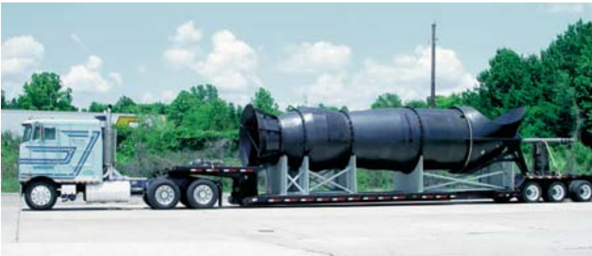
5 After extensive repair and upgrading, one of twelve cooling water pumps is transported back to the customer.
