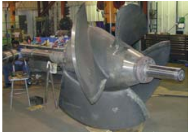
4 A semi-axial flow vertical impeller assembled on shaft is ready for pump assembly.
