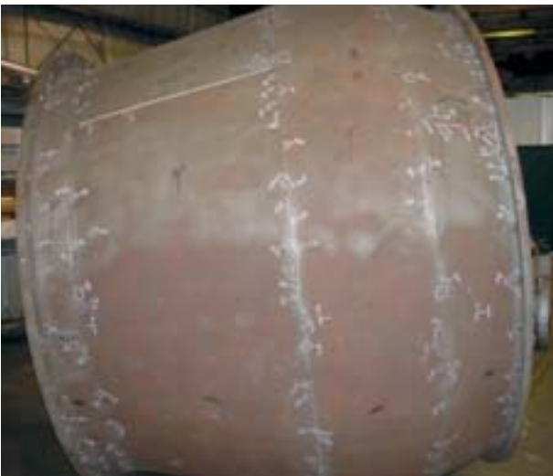
2 When upgrading a cooling water pump to nuclear-safety standards, much attention was paid to the identification of weld defects, using non-destructive examination techniques.
