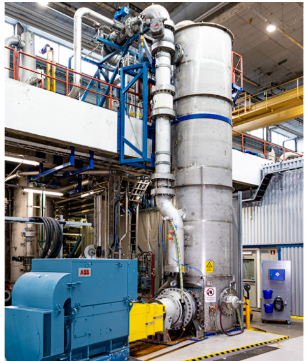
The world's biggest MCE pump is being tested in Sulzer's research and development center
