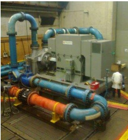
Performance test of the customer's new unit in a Sulzer factory in England
