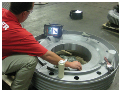
Phased array UT inspection
