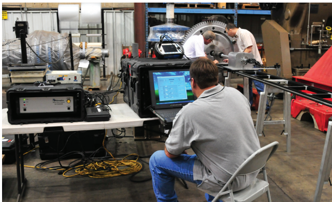
Boresonic inspection of a turbine disk
